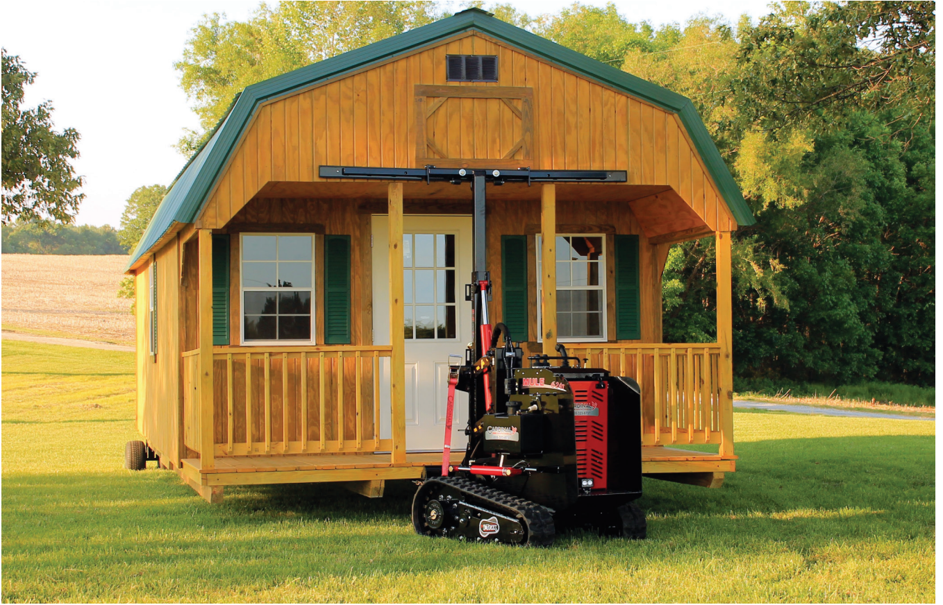
A mule makes the job of maneuvering a shed easier. PHOTO COURTESY OF CARDINAL MANUFACTURING
