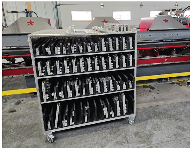
The Star 1 Products air over hydraulics long folder. Shown below: Each template holds the key to creating a different trim profile. PHOTOS COURTESY OF STAR 1 PRODUCTS.
