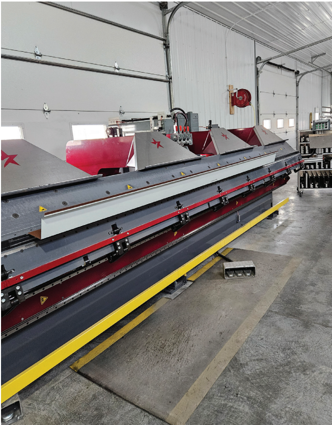
The template system with pneumatic controls makes bending quick and accurate.
