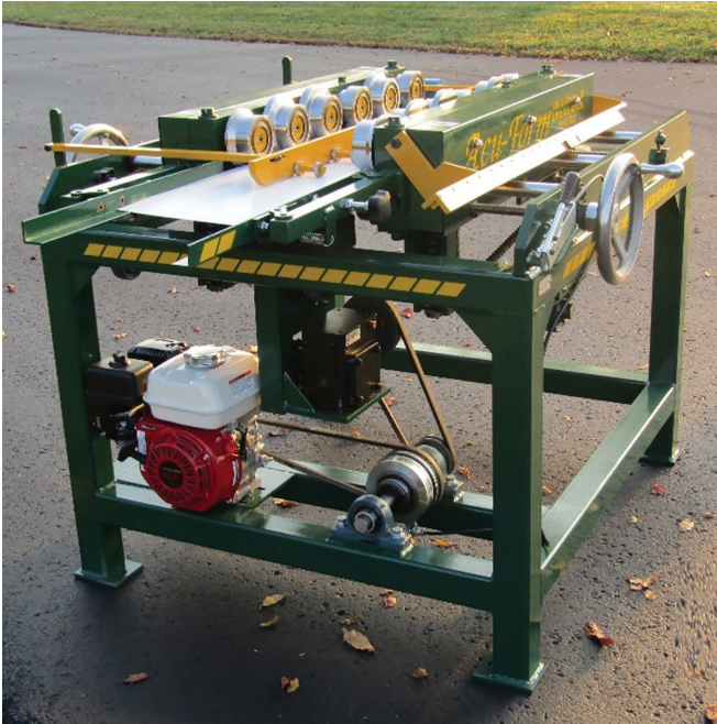
A gas-powered hemming machine from Acu-Form. PHOTO COURTESY ACU-FORM EQUIPMENT.
