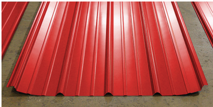
Fig 1: Panel with underlayment formed with typical standard tooling.
