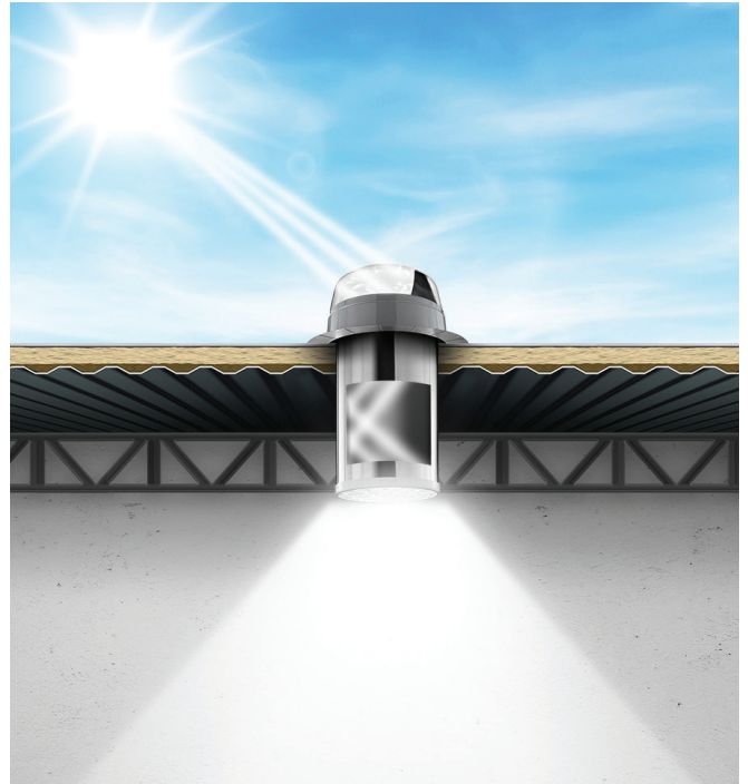
Tubular daylighting selectively captures sunlight, stripping it of ultraviolet light and heat, and redistributes it. PHOTO COURTESY OF KINGSPAN LIGHT + AIR NORTH AMERICA
