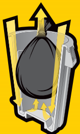
BUILT IN VENTING CHANNELS
